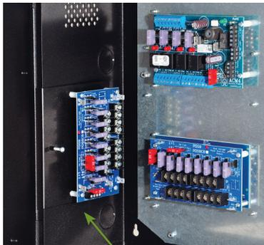
BR1 with sub-assembly (not included) mounted to side wall of Trove Enclosure.
